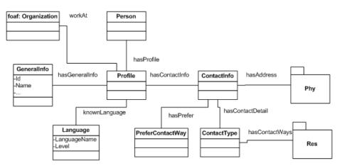
Figure 3.2: User profile package UML diagram
