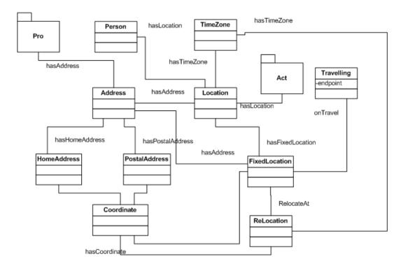
Figure 3.5: Physical environment package UML diagram
